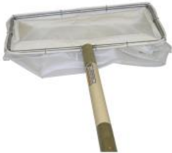
Figure 6.2 Standard kick net (500 \mu m) used for collecting benthic macroinvertebrates.
